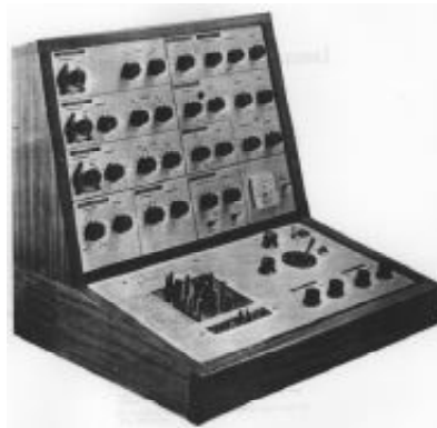
Fig. 7. A 1970 VCS-3 Putney. Although a small keyboard could be attached to it, it was often played by turning knobs.
