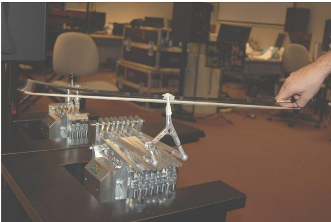
**Fig. A.1** The TGR device in 2-DOF configuration with a bow attached. We did not use this configuration for testing, however a simple, not-very-robust coupling using tape was attempted briefly to explore how a bow would feel when attached to the device.
