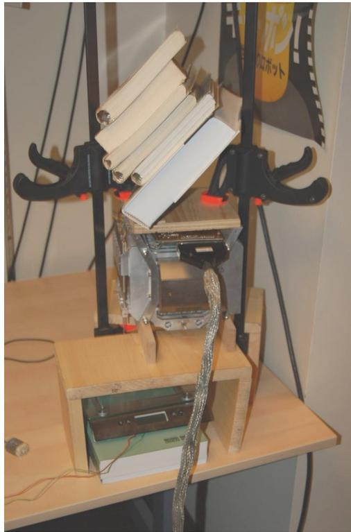
**Fig. A.2** The device calibration setup. The device is upside-down balanced on two blocks, with clamps used to ensure that the blocks do not tip. A rod attached to the motor pushed on an electronic kitchen scale. Heavy books are piled on top to ensure the device, which was not clamped to the desk itself, does not move upwards when exerted downward pressure on the scale.
